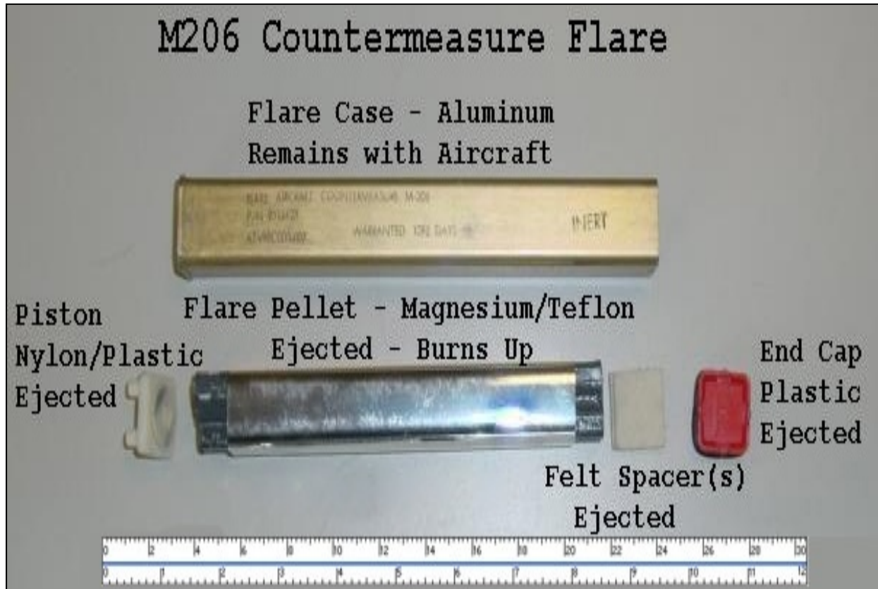
Figure 7–2. Photograph of M-206 Flare Components
