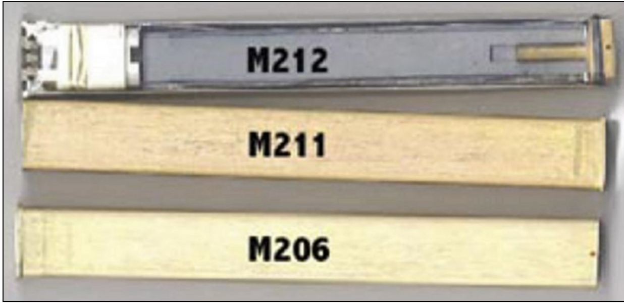
Figure 7–12. M-211 and M-212 Flares Developed to Respond to New Threats with M-206 Flare for Reference
